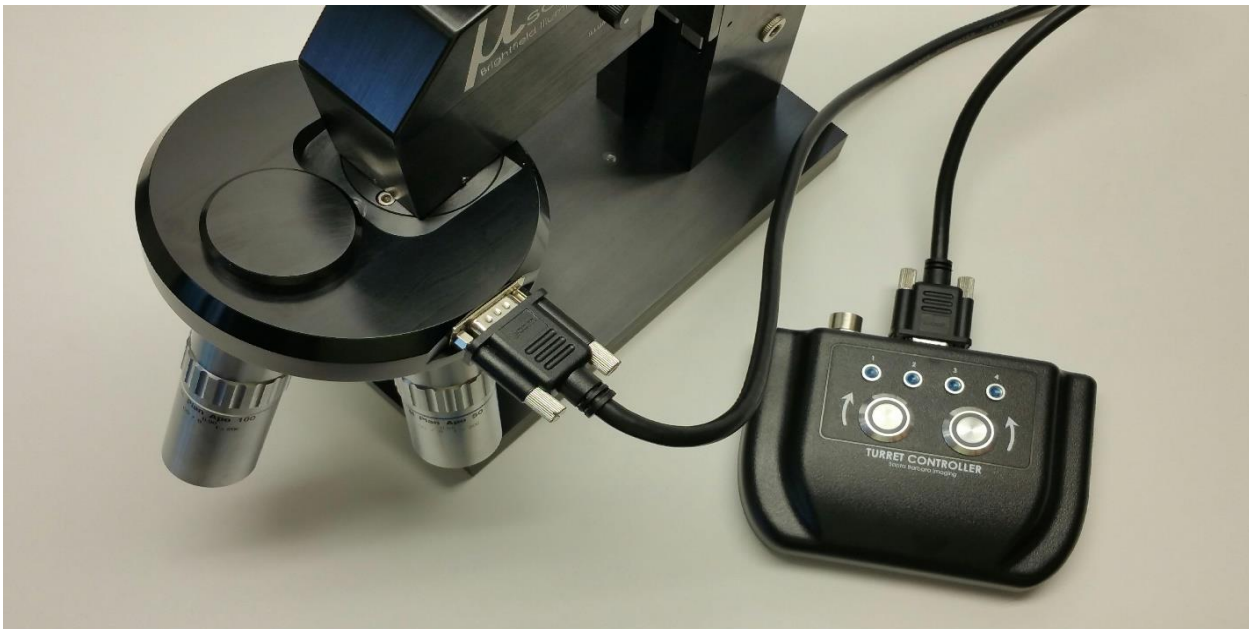
Top View of Motorized Microscope Turret Mounted on Santa Barbara Imaging's uScope
