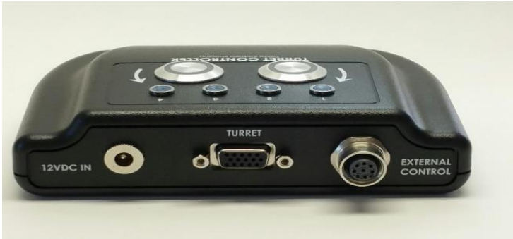
View of Controller Connections Panel
